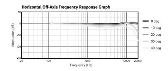
Frequency response is measured on-axis at a distance referenced back to 1m at 1-watt drive. Shown as half-space ( $2\pi$ ) environment.
